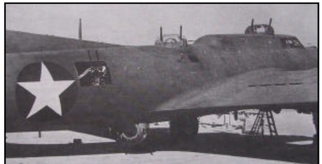
Fuselage detail of a YB-40 showing twin gun waist Position installation and the second, mid-fuselage, dorsal turret
