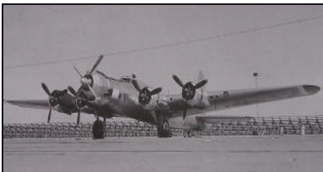
The Curtiss-Wright testbed mounted a reciprocating R-3350 engine in the centre location.
