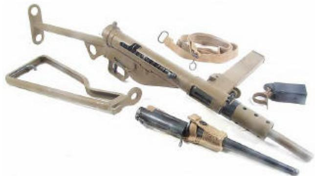
Mk 2 Sten showing the two types of shoulder stock, bayonet, sling and magazine loading tool
